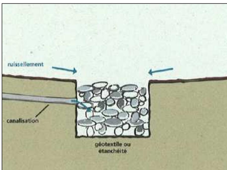
SCHEMA DE PRINCIPE – BASSIN DE RETENTION
